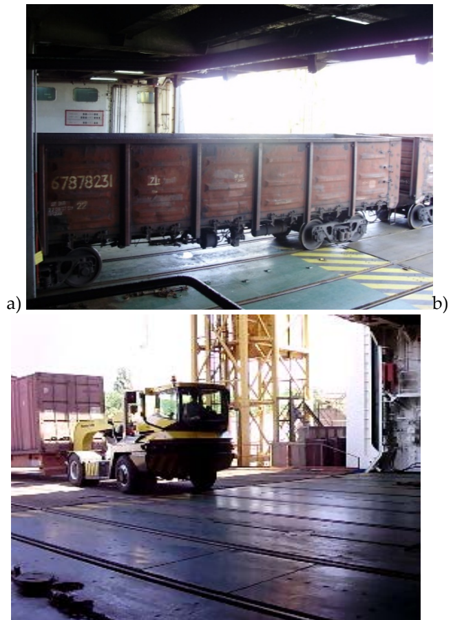
Figure 2. Loading of railway vehicles on train ferry a) Heroes of Shipka; b) Greifswald
