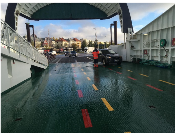
Figure 9. Loading and stowing vehicles in Molde ferry terminal. Designated area for dangerous goods is thoroughly marked on the deck, using red paint.
