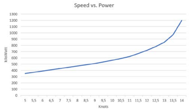
Figure 5. Combined power demand on the propulsion equipment at different velocities [8].
