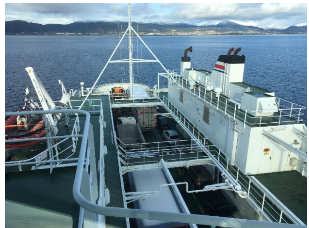
Figure 10. Example of one limitation where heavy cargo is placed in the bow, potentially slowing down unloading operations.
